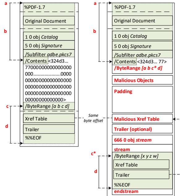
**Figure 9: A comparison of the original document and the manipulated document by using the Signature Wrapping Attack (SWA). Malicious objects are placed before the malicious *Xref table* by deleting unused zero bytes in *Contents*.**
