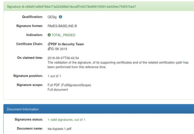
Figure 11: Validation report created by the Digital Signing Service for a manipulated but signed PDF file [14].
